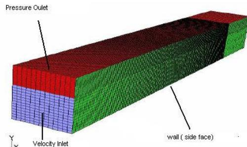
Figure 1: Test tank domain with boundaries applied.
