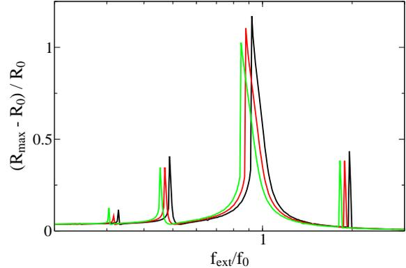
Figure 4: Frequency response (from right to left) for —  $N_{bub} = 1$ , —  $N_{bub} = 2$ , —  $N_{bub} = 3$ , near a rigid boundary, without time delay ( $R_0 = 100 \mu\text{m}$ ,  $D = 1.2 \text{ mm}$ ,  $r = 2 \text{ mm}$ ).
