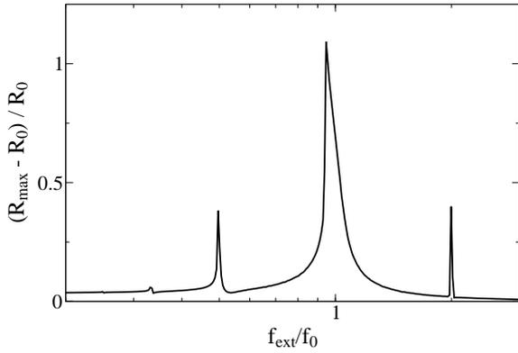
Figure 2: Frequency response for a single bubble ( $N_{bub} = 1$ ,  $R_0 = 100 \mu\text{m}$ ) in an unbounded domain ( $D = \infty$ ,  $r = \infty$ ), without time delay.
