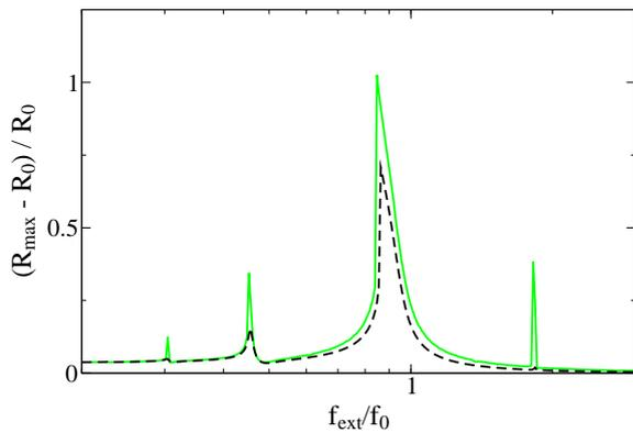
Figure 6: Frequency response for  $N_{bub} = 3$  near a wall ( $R_0 = 100 \mu\text{m}$ ,  $D = 1.2 \text{ mm}$ ,  $r = 2 \text{ mm}$ ). — without time delay, ---- with time delay.
