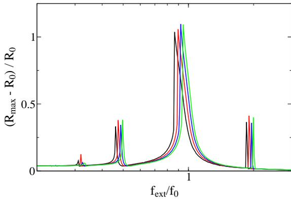
Figure 3: Frequency response for a single bubble ( $R_0 = 100 \mu\text{m}$ ) without time delay, with varying separation distance to a rigid boundary. From left to right: —  $D = 3R_0$ , —  $D = 5R_0$ , —  $D = 10R_0$ , —  $D = 50R_0$ .
