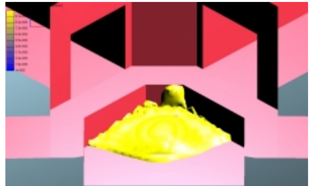
Fig. 14 Dust iso-contours or iso-surface ( 100\text{mg}/\text{m}^3 ) (full bin scenario) (steady state case)
