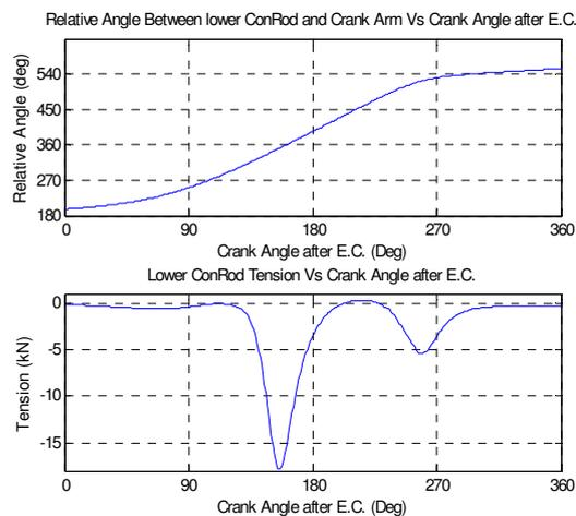
Figure 7. Thermodynamic model results used to specify the FEA loads.
