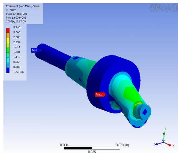
Figure 8. FEA stress contour plots of the crankshaft
