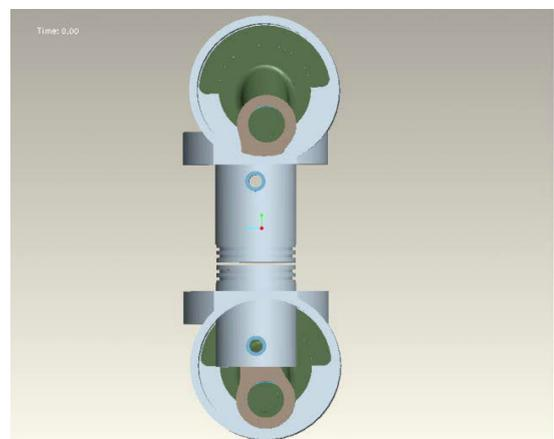
Figure 5. ProE display of the prototype solid model with the cranks located at a position just before the start of the induction stroke – crankshafts rotate clockwise as viewed. The image shows that the upper crank lags the lower crank by a few degrees. Crank offsets results in asymmetric piston motion between the 'up' and 'down' strokes creating the displacement depicted in Figure 1.
