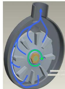
Figure 8: Pump throat area / impeller outlet area Ratio
