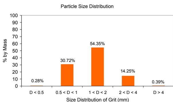
Figure 11: Particle size distribution for grit used to artificially roughen the test plate.
