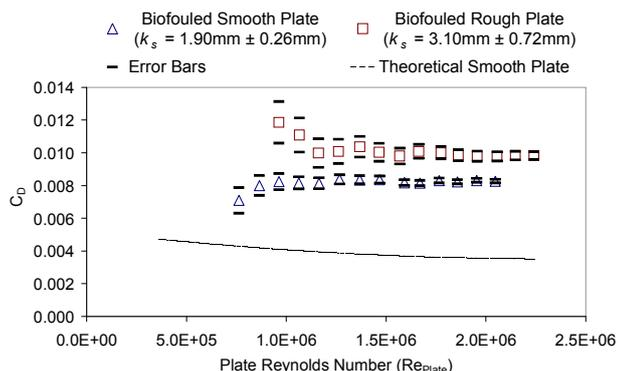
Figure 12: Total drag results for biofouled test plates.
