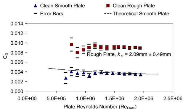
Figure 10: Total drag results for clean test plates.
