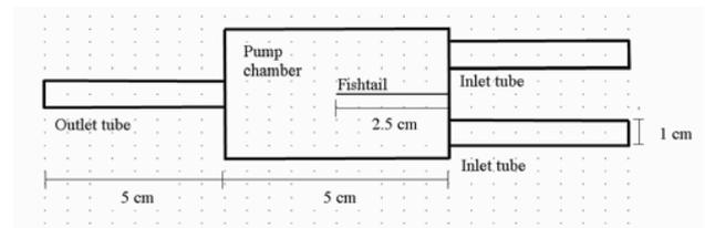
Figure 4. Diagram of the trilayer strip "fishtail" actuator.
