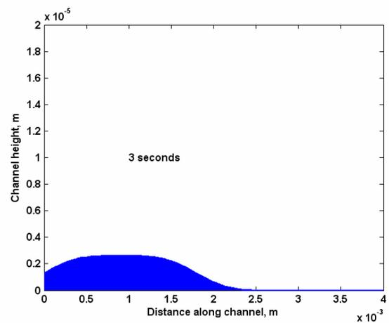
Figure 1. Deformation of a polymer film causing flow along a microchannel.
