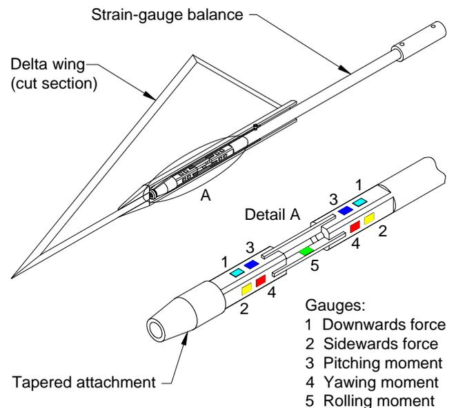
Figure 6. Five-component strain-gauge balance
