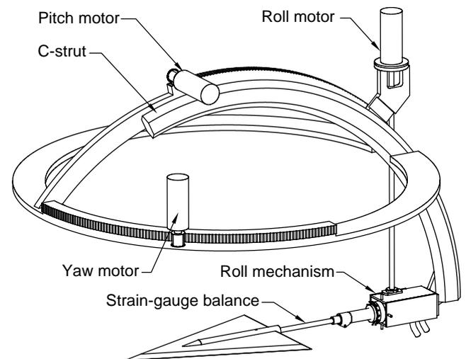
Figure 3. Diagrammatic representation of upgraded model motion system.
