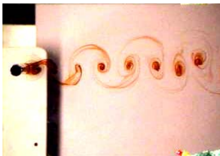
Figure 2: Flow visualisation of the von Karman vortex street produced by forced flow behind a cylinder in cross flow.
