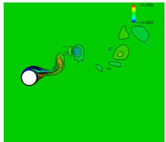
Figure 4: Contours of vorticity around a rotating cylinder at Re=10^3 , \alpha = 2.0 .
