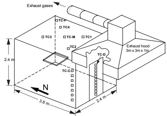
Figure 1. Schematic diagram of ISO 9705 fire test room
