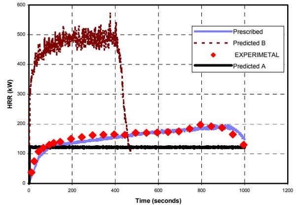
Figure 2. HRR profiles from FDS and experimental results
