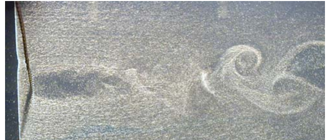
Figure 1: Hydrogen bubble flow visualisation of structures behind a grid (from [4]).
