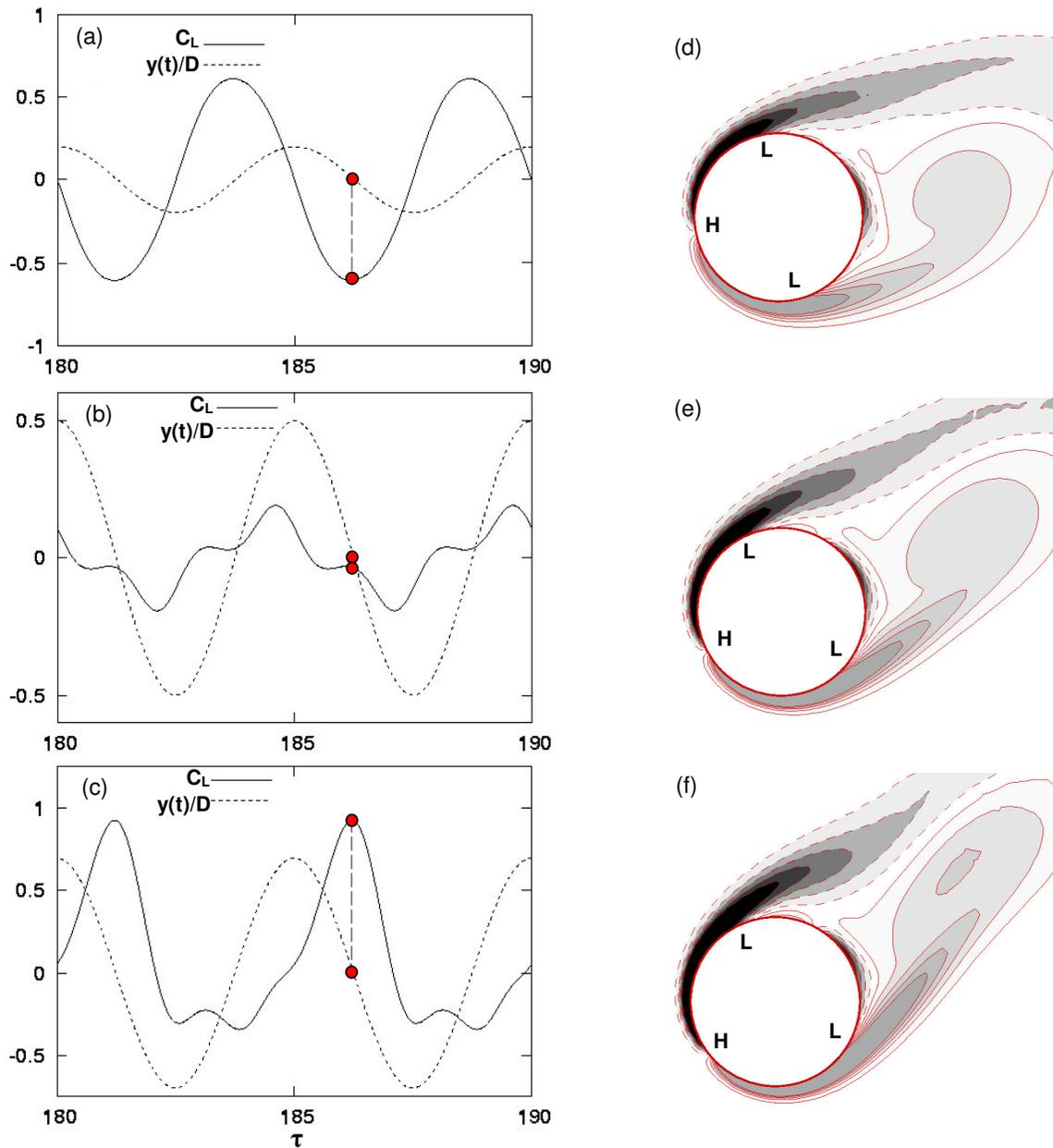
Figure 2. Lift coefficients and corresponding vorticity contours for cylinder oscillating at  $V_i=5.0$ , (a)  $A/D=0.199$ , (b)  $A/D=0.497$  and (c)  $A/D=0.696$ . Red dots indicate point at which images were obtained. Negative vorticity is shown in black and enclosed by dashed contours. H and L show high and low pressure regions respectively.
