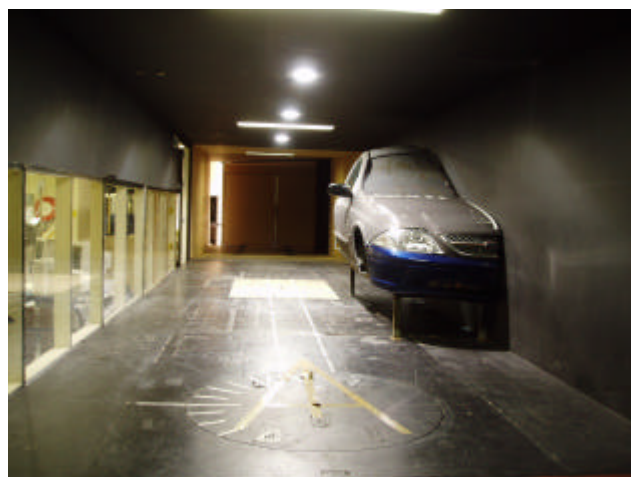
Figure 2: Experimental Set Up of the Mirror with a Ford Quarter Model in the Test Section of RMIT Wind Tunnel.
