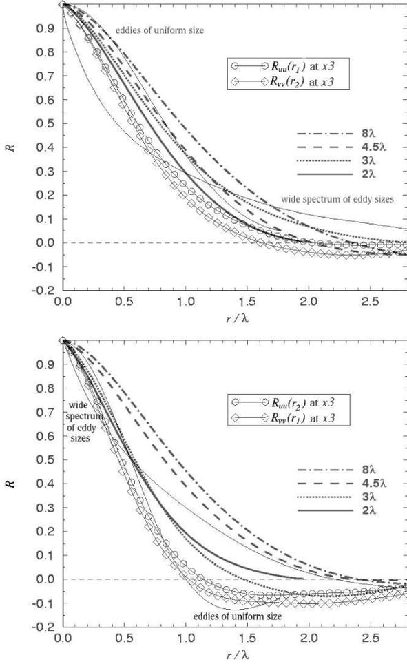
Figure 1: Longitudinal and transverse velocity autocorrelation functions obtained from DNS data by progressively restricting the spatial domain ( $Re_\lambda = 26$ ) compared to experimental data obtained using a spatial domain of  $3\lambda$  ( $Re_\lambda = 23$ ). Top: longitudinal autocorrelation; bottom: transverse autocorrelation.
