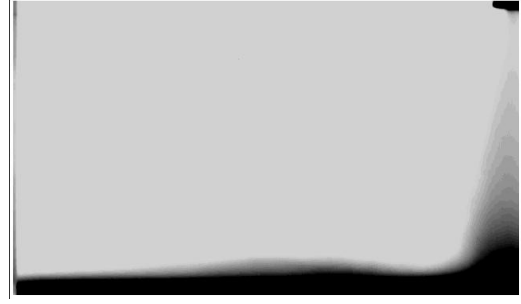
Figure 3: Time-averaged image of the outflow showing the radial growth in thickness near the source and adjustment to a constant thickness gravity current. The right-hand boundary of the image is the plume centreline. The outflow is the horizontal dark grey region.
