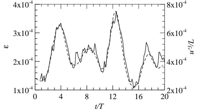
Figure 3: Example of the offset time series for Run E ( $\tau_{\max}^+ \approx 0.74$ ),  $N = 256^3$ , average  $Re_\lambda \approx 150$ . Note that the peak events are now well correlated. —,  $u'^3/L(t/T)$ ; - - -,  $\varepsilon([t - \tau_{\max}]/T)$ .
