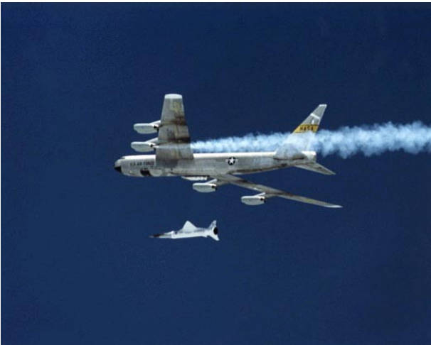
Figure 9: Moments after release from NASA's B-52 carrier aircraft, X-43A/Pegasus "stack" is seen before ignition of the Pegasus rocket motor (June 2, 2001). Image from NASA/Dryden Flight Research Center Photo Collection.
