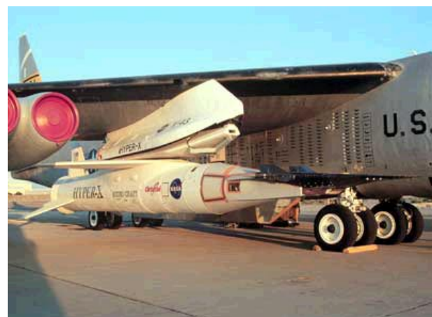
Figure 8: X-43A/Pegasus “stack” shown attached to its B-52 carrier aircraft . Image from NASA/Dryden Flight Research Center Photo Collection.
