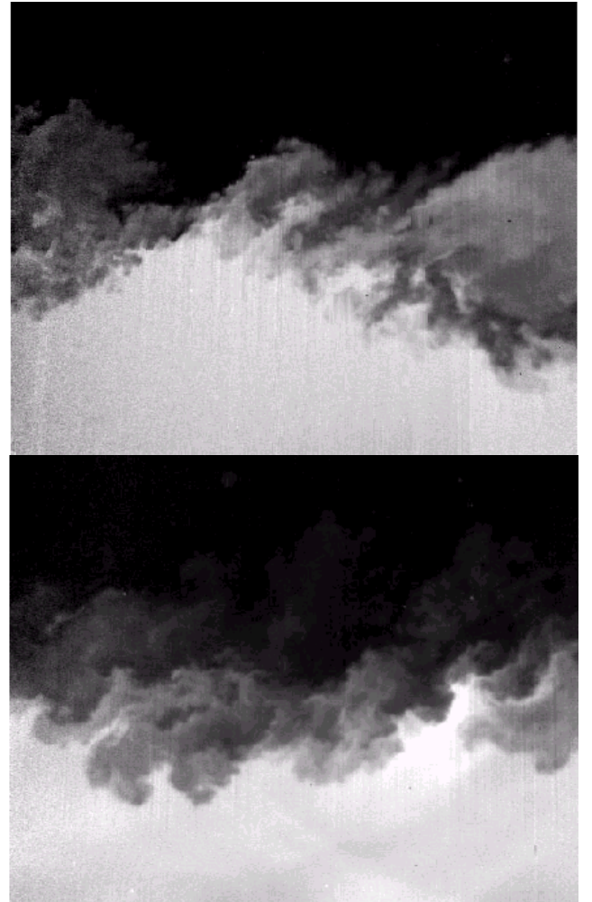
Figure 11 Rayleigh-scattering images of high- Re shear layers [18]. Top: Low-compressibility flow ( M_c = 0.15 ), U_1 = 200 m/s [ N_2 ], U_2 = 100 m/s [ C_2H_4 ]. Bottom: High-compressibility flow ( M_c = 0.96 ), U_1 = 1150 m/s [ He ], U_2 = 100 m/s [ C_2H_4 ].
