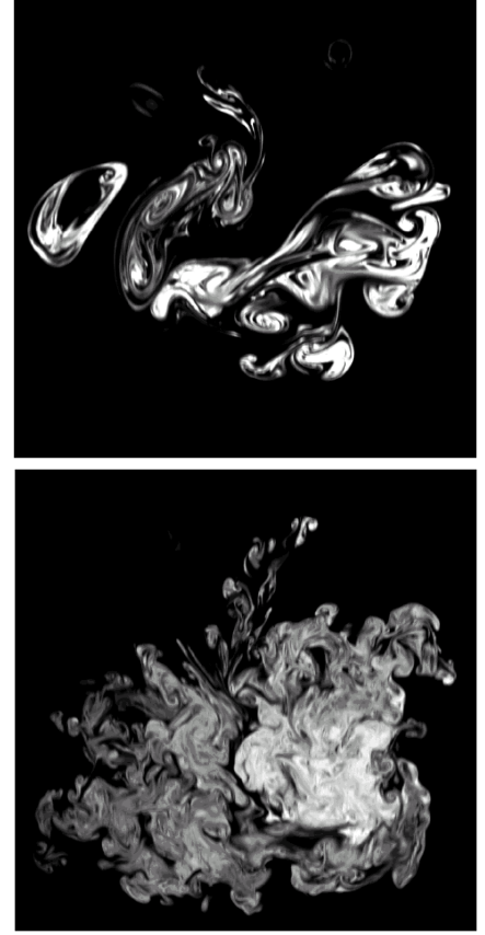
Figure 7 Jet-fluid concentration for a transverse jet in a uniform freestream (cf. figure 2), at x / d_j = 50 . Top: Re = 1000 . Bottom: Re = 10,000 [6].
