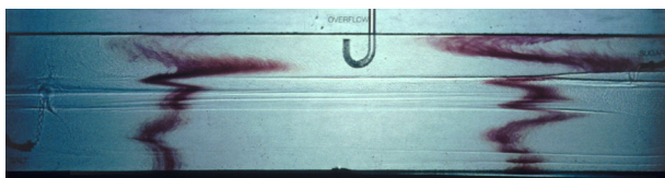
Figure 1. Shadowgraph of the layers formed in an experiment with separated salt and sugar sources; dye streaks added to show the shears.
