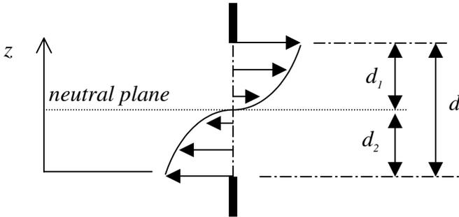
Figure 3 Schematic of natural convection across a vertical opening
