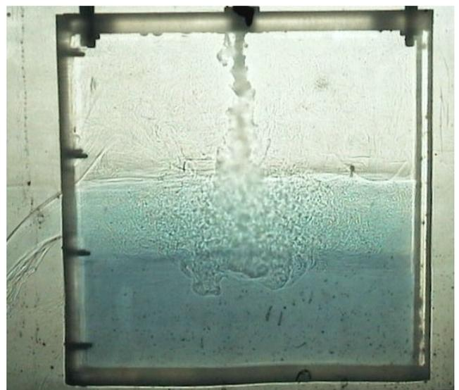
Figure 8. Shadowgraph of the ventilated enclosure of figure 6 in a transient state following a substantial reduction in the strength of the buoyancy source.
