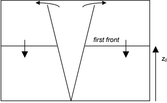
Figure 2 Turbulent buoyant plume rising into a sealed, adiabatic space generating a stratified environment.
