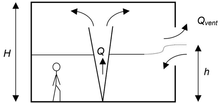
Figure 4 Enclosure with a point source of buoyancy and a vertical opening at a height  $h$  above floor illustrating flow with the *critical* vent area,  $A_{crit}$ , required to ensure buoyant layer remains above opening
