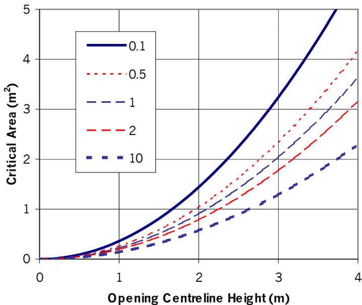
Figure 5. Plot of the critical vent area required to maintain the buoyant, contaminated layer above the mid-height of the enclosure opening with vent aspect ratio,  $\gamma$ , taking values of 0.1, 0.5, 1, 2 and 10.
