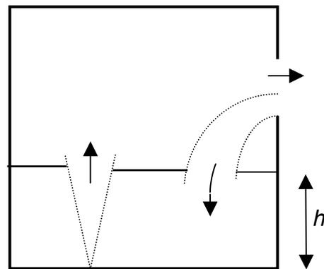
Figure 7. Schematic of flow modelled by Linden *et al.* [7] for  $A_{vent}/A_{crit} \ll 1$  where exchange flow through opening generates a descending plume that feeds a mixed layer in the bottom of the enclosure.
