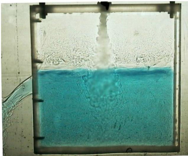
Figure 6. Shadowgraph of steady state experiment with single, square opening ( $\gamma = 1$ ) in the left hand sidewall of the enclosure  $A_{vent}/A_{crit} = 0.79$ .
