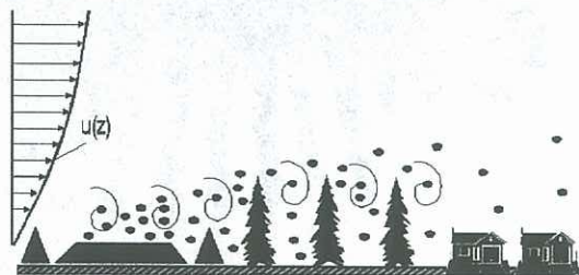
Figure 1: Principle sketch of the ground deposition after particle erosion from a bulk pile.
