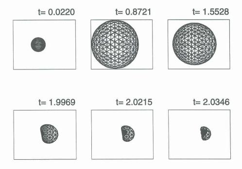
Figure 2: The growth and collapse of a cavitation bubble for  $\gamma = 1.5$ ,  $\delta = 0.1$ . The wall position is given by the right hand side of the frame.
