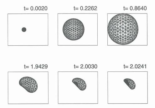
Figure 1: The growth and collapse of a cavitation bubble for  $\gamma = 1.5$ ,  $\delta = 0.25$ . The wall position is given by the right hand side of the frame.
