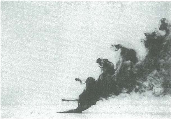
Figure 7. Flow pattern obtained when dye is injected from the circumferential slot and the dye injection port at R = 2.2 and Re = 1,600 .
