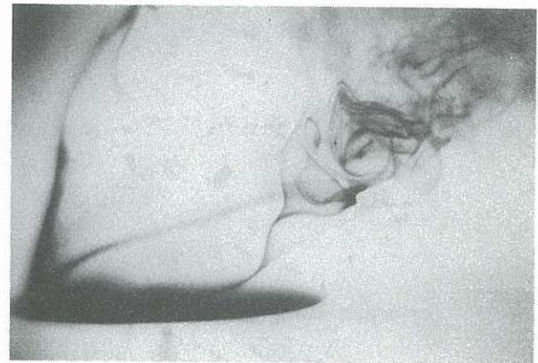
Figure 4. Close-up view of vortex breakdown in the scroll-like roll-up of the shear layer at R = 4.0 and Re = 1,600 .
