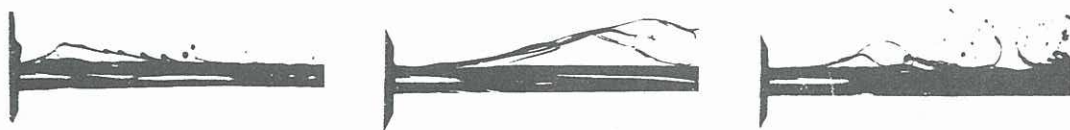
Fig. 6 - Ethanol jet, D = 200 \mu\text{m} , V = 12 \text{ m/s} , P_\infty = 100 \text{ Pa} , P_s = 5.9 \text{ kPa}
