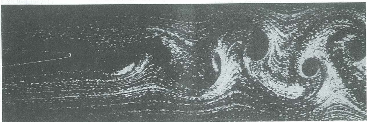
Figure 1. Vortex shedding from a symmetrical Aerofoil, Re_{chord} 15000 , incidence 4 deg
