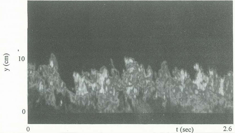
Figure 2. Color-enhanced reproduction of flow in plume-mixing regime (red indicates a value of C/C_0 = 0.1 )
