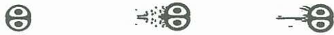
Fig.2 Contour plots of entropy for an unperturbed Lamb dipole at (a) t = 0. , (b) t = 11. , (c) t = 96.
