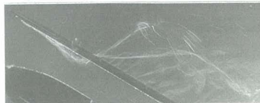
Fig.6 Apex lower surface vortex and wing vortex ( h/c=-0.1 ; l/c=0.05 ; \alpha=30^\circ ; R=5.2 \times 10^4 )
