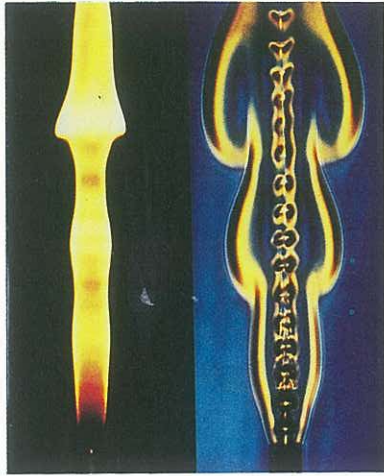
Figure 1 Typical propane diffusion flame and schlieren image.
