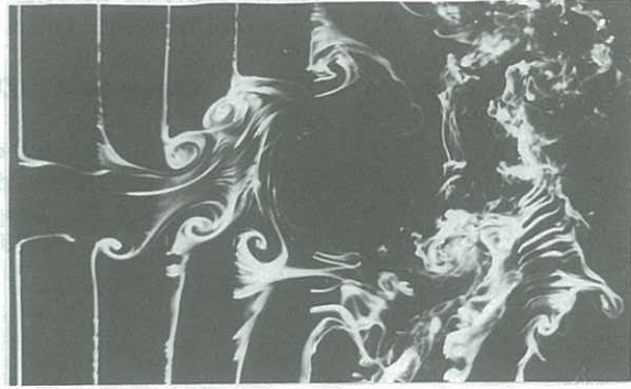
Fig. 3 Instantaneous flow pattern at phase (vii) visualized by smoke.
