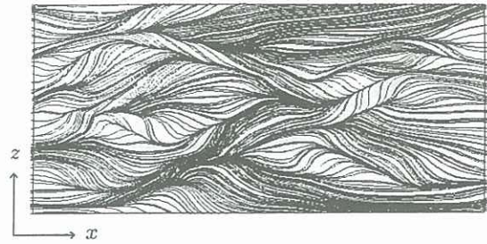
Fig. 11 Wall streamline pattern in a turbulent wall flow computed by Moin and Spalart.
