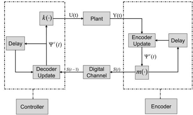
Fig. 1. Dynamic quantised control scheme.
