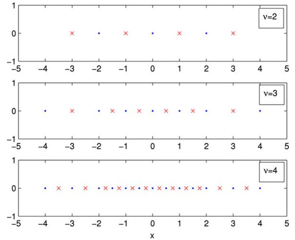
Fig. 2. Quantiser points and intervals ( $\mu = 2$ ). Boundary points and quantiser points are denoted by 'x' and '.' respectively.
